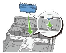
2 Insert the retard roller into the axle until it snaps. The protrusions fit completely into the slots and the roller hook reseats into the groove on the axle.
